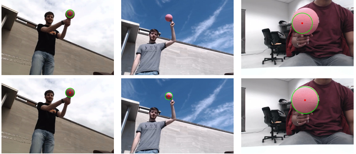
Figure 4.4: Comparison of ball detection results displayed on original frame using HSV (top) and SVM (bottom) background segmentation.
